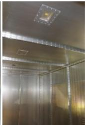
Electromagnetic reverberation chamber is a multifunctional **EMC** (Electromagnetic Compatibility) test facility for commercial, military, automotive testing and other electromagnetic investigations.
