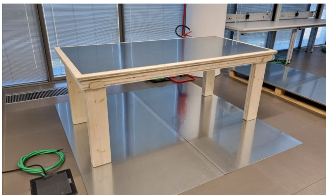
Test Table for CISPR 25
